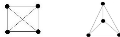
(a) Regular K_4 graph (b) Embedding of K_4 in the finite plane
